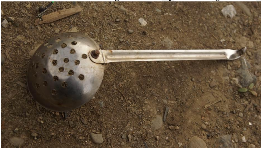
Figure 5. A tool used during winter fishery for cleaning an ice-hole from ice. Pobedino, Sakhalin Island. September 2014 (photo made by V. Davydov).
