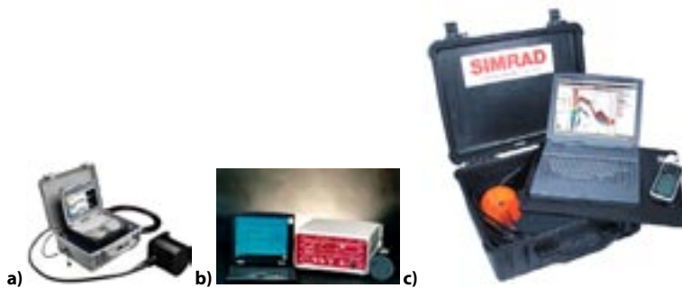
FIGURE 2. — Portable split-beam hydroacoustic systems from the major manufacturers: (a) Biosonics Inc., (b) Hydroacoustic Technology, Inc. (HTI), and (c) Simrad. Systems include an echo sounder contained in a rugged container or rack-mountable unit that has waterproof ports for attaching transducer cables, global positioning system cables, and network cables. Systems are controlled via wired or wireless LAN communication by a laptop computer.
