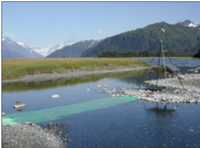
FIGURE 1. — Video camera set up on tower in an Alaskan river (note contrasting panels on river bottom).
