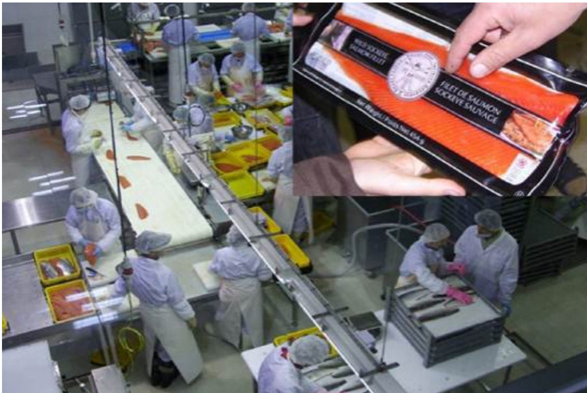
Figure 2. Vacuum packing section of the Vityaz-Avto fish processing facility and an example of its production.
